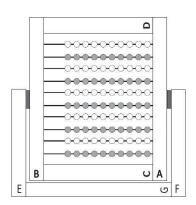
Apply glue on the ends of E and F screw them into G to form a flat-bottomed 'U" shape. Sandwich the washers between the upper sides of the 'U" shape and the holes in the middle of A and B. Attach with screws.
